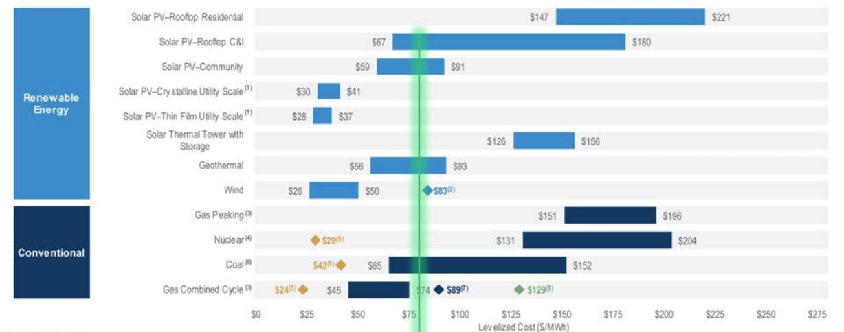
Selected renewable energy generation technologies are cost-competitive with conventional generation technologies under certain circumstances
